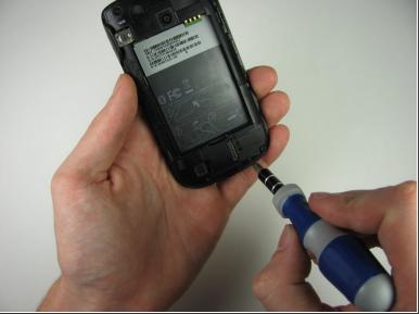
Remove the four 4.9mm T6 Torx screws that secure the back panel to the rest of the phone.
