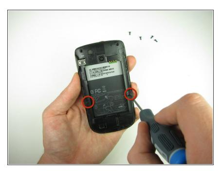
Remove the two 4.3mm Phillips #00 screws that secure the back panel to the rest of the phone.
