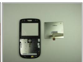
Pry the LCD screen out by using the plastic opening tool or your fingers.
