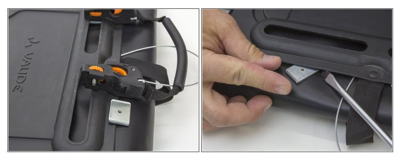
• Slightly lift the hardback panel using a screwdriver and push the thread place underneath.
