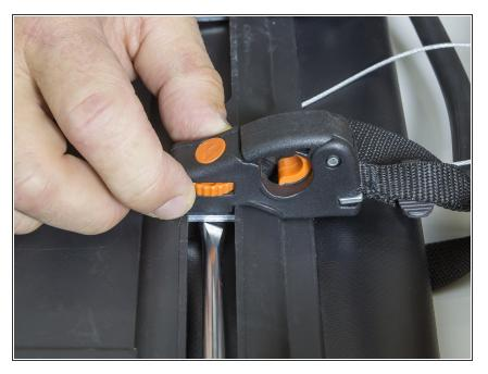
Position the QMR hook on the thread plate. Attach the screw to the thread plate using the orange knob.
