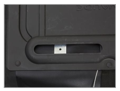
• Adjust the thread plate in the middle of the groove.
