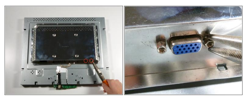
Using a nut driver (or if necessary, needle-nose pliers), remove the two nuts on either side of the VGA input.
