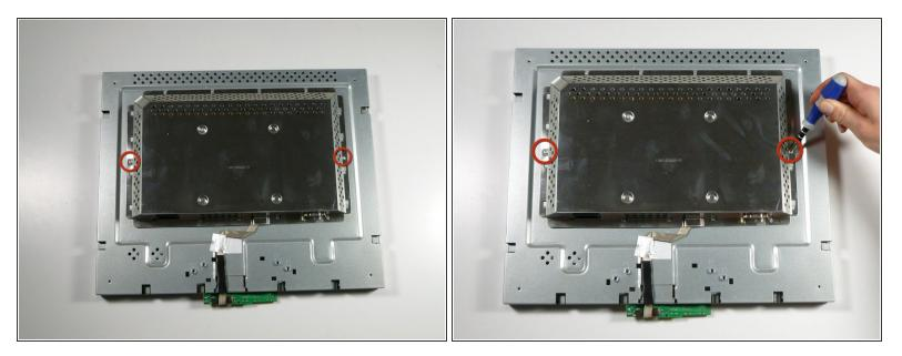
Remove the two 5.7 mm Phillips #2 screws located on either side of the EMI shield.
