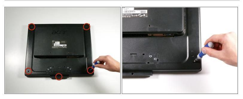
• Remove the five 9.5 mm Phillips #2 screws located around the perimeter of the monitor.
