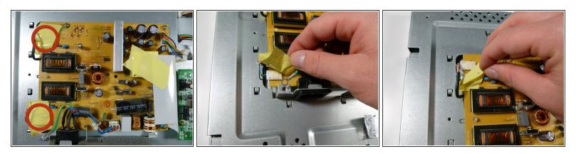
Remove the two pieces of yellow tape on the left side of the power supply.
