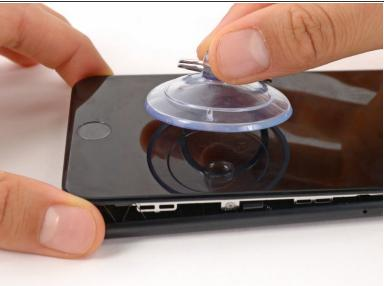
Pull up on the small nub on the suction cup to remove it from the front panel.
