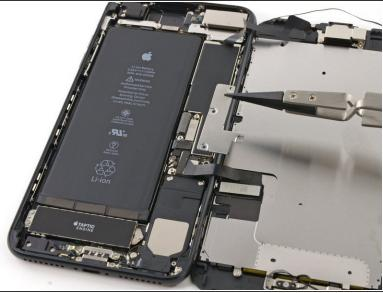
Remove the lower display cable bracket.
