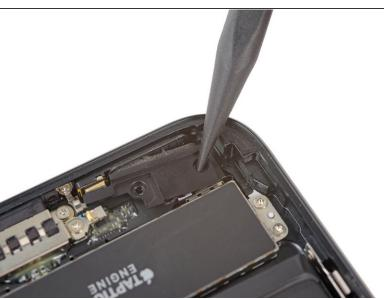
Gently push the barometric vent in the direction of the Taptic Engine to separate the adhesive securing it to the bottom edge of the iPhone.
