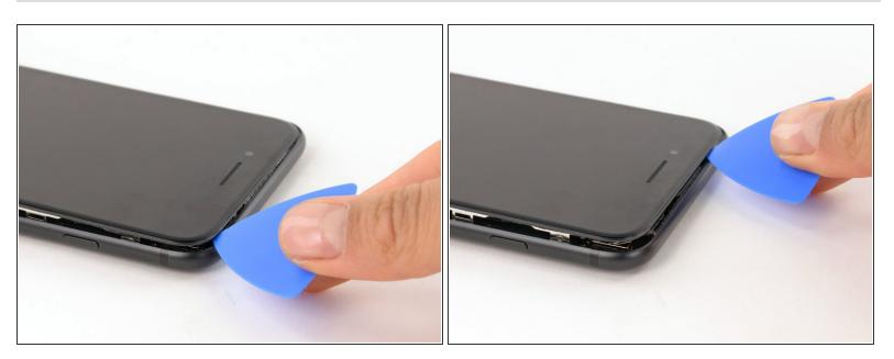
Slide an opening pick underneath the display along the top edge of the phone to loosen the last of the adhesive.
