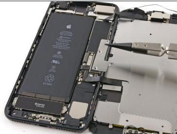
• Remove the lower display cable bracket.
