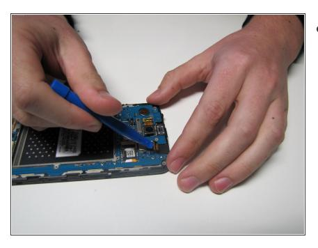
With tweezers remove the front facing camera piece on the motherboard, and insert the new piece in the position of the old one.
