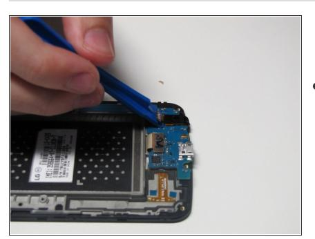
With tweezers remove the headphone jack piece on the motherboard, and insert the new piece in the position of the old one.
