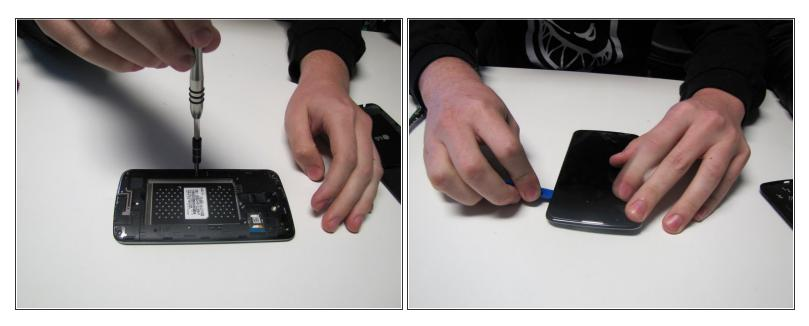
Unscrew every screw of the bottom of the phone and use guitar picks to remove the plastic frame of the phone
