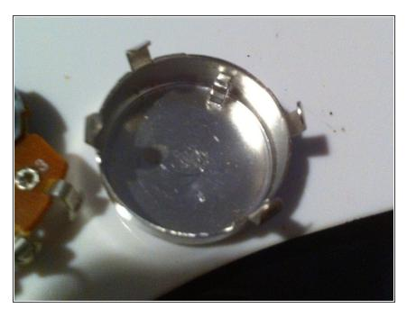
You are ready to put it back into the back of the pot. Note the tab inside the metal pot backing. You'll have to put it back in the same alignment that it was in before disassembly. also the plastic tab on the black plastic piece will need to go to either side of the metal tab otherwise you won't be able to put the metal backing on. See next.
