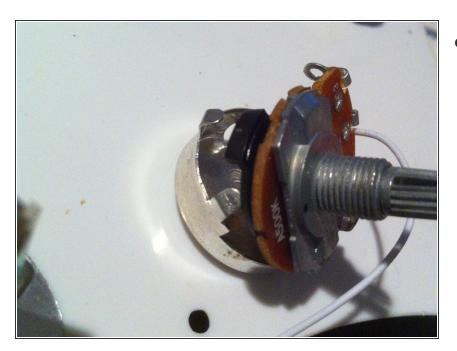
Phere you see the black tab previously mentioned. Put the two pieces together that you see in the photo in the same alignment that they were before disassembly. Turn the stem either to the left or right so the metal tab in the backing and the black tab are not directly on top of one another and everything should go together tightly. See next.
