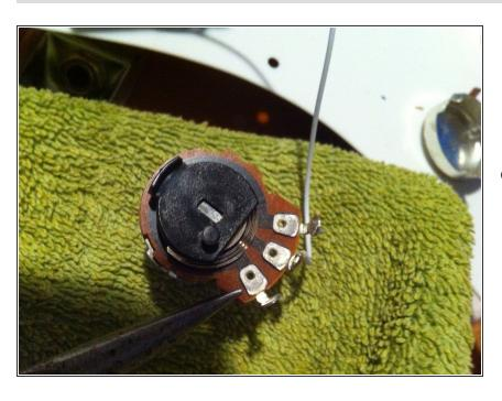
Find a hard surface to do the next step on. I used a cloth to help stabilize the pot. Note the end of the slotted stem inside the hole of the black plastic piece. It is correctly lined up and just beginning to go into the hole. It will fit very tightly. use a finger to press down more while keeping everything aligned. Takes a lot of pressure.
