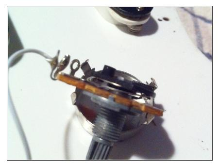
• Here the metal stem holder is properly aligned with the fiberboard. This is important because all three pieces must be aligned in order for it to go back together completely. Carefully align the hole in the black plastic piece with the slot on the end of the stem and get it started by pressing down on the black piece till it begins to go together.
