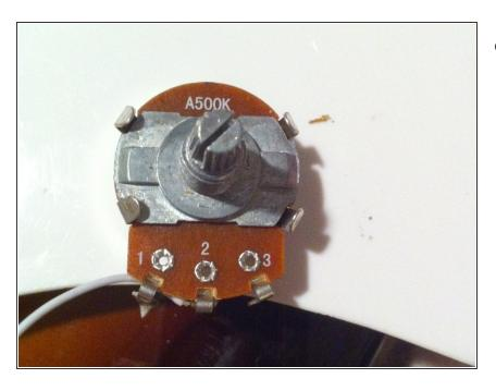
Once you have removed the affected pot (potentiometer) from the guitar, set it on a stable surface. Take photos or make note of how everything fits together so you put it all back together the same way. I also made marks to help. Bend back the tabs that hold it together as shown in the photo.
