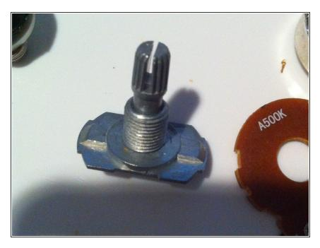
Start the reassembly process by inserting the stem with the knurled knob end up.
