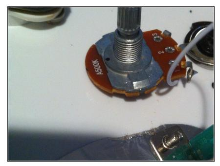
Put the metal stem holder piece on top of the brown fiberboard piece aligning them in the process. Be sure to align them in the same orientation that they were in before disassembly. Refer to your starting photos or diagrams.
