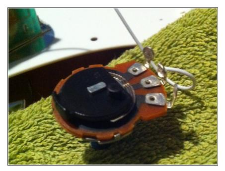
Take you time and work it gradually until the end of the stem is well inserted in the hole of the black plastic piece. Keep checking to see that all three pieces are still properly aligned. Note that now the stem is more visible above the surface of the black plastic and all 3 pieces are still aligned correctly. At this point it is assembled.
