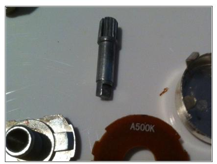
You now have all the pieces laid out. Note that the stem has a slot end that is the same shape as the hole in the loose piece (made of black plastic in the previous photo.
