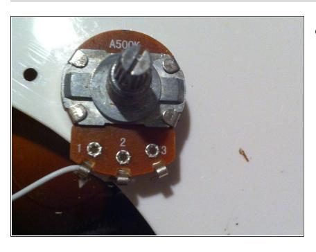
Here you see that the tabs have been bent back to the position that they were before disassembly and the pot is now reassembled!
