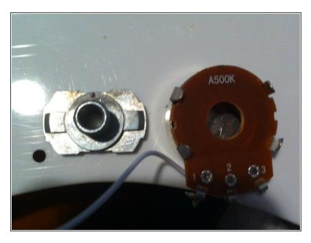
Make note of how it is positioned then lift off the metal stem holder.
