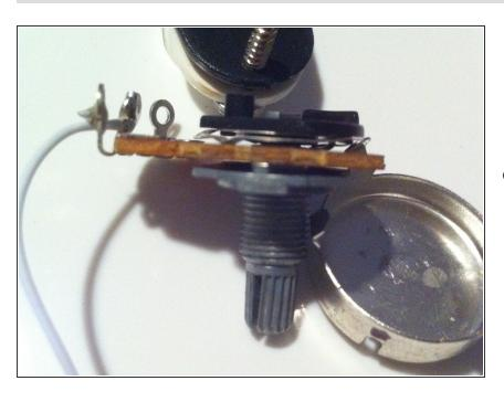
Next start to align the loose piece (black plastic) over the end of the stem. You will have to align the hole in the black plastic piece with the end of the stem. The brown fiberboard piece must be in between at this point. Also note how the small tab on the metal stem holder is not quite matching up with its slot in the fiberboard. See next photo
