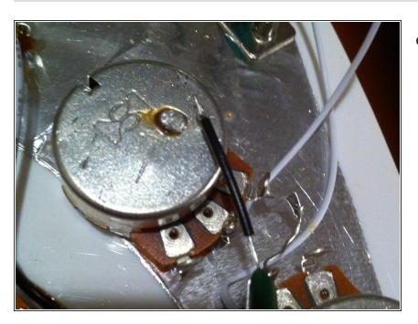
Replace the pot back into the guitar pickguard so it is in its proper alignment on the guitar. Begin to reattach any de-soldered connections. Mine needed two wires reattached. Put yours back together so they are the same as they were before you began disassembly. Refer to your initial photos or diagram.
