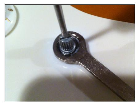
Carefully attach your reassembled pot to the guitar and gently tighten but don't over tighten. Be sure the pot does not twist out of position while you are doing this.
