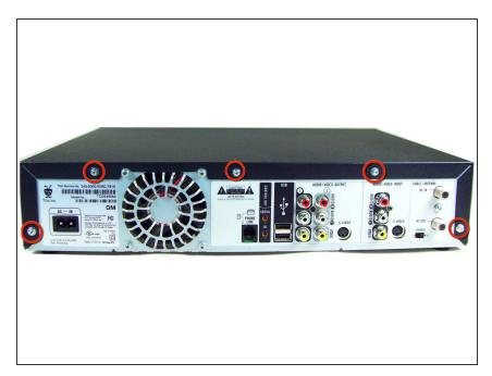
Unscrew the five 0.31 inch T-9 screws on the back cover.
