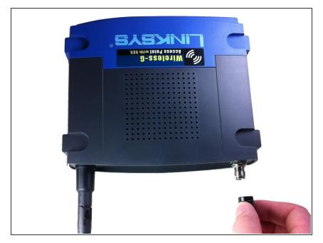
Once antenna is completely detached, obtain the new antenna, and place it on device so the threads line up.
