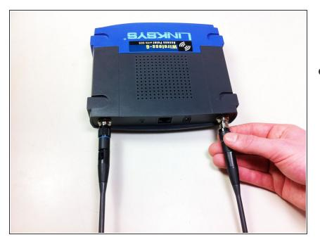
Grip antenna at the base and twist counter-clockwise to unscrew it from the device. The base should have a rough feel to it.
