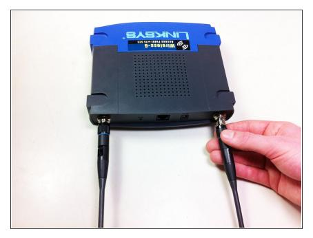
Screw antenna onto device by twisting the base of the antenna in a clockwise motion until it is tight and does not turn any further.
