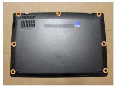
Loosen the seven cover screws.
