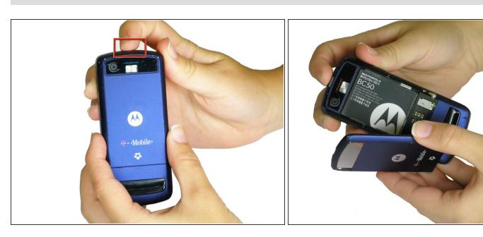
Press the panel release button on the top of the phone and simultaneously pull the rear panel away from the phone.
