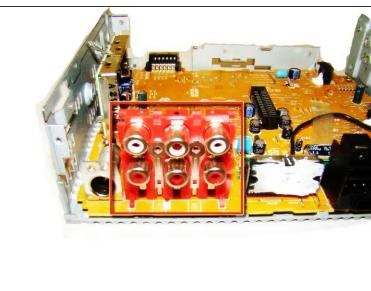
To remove the Audio In/Audio Out inputs on the circuit board please refer to the <u>iFixit soldering</u> guide to assist you.
