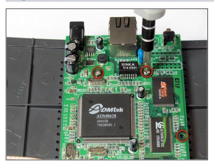
Using a Phillips screwdriver remove the the three screws that fasten the main circuit board to the chassis.
