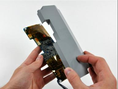
If you wish to replace just the inverter board, use a spudger to pry off its plastic cover.
