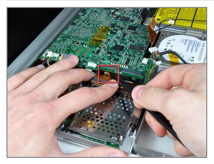
Lift the left side of the logic board and disconnect the modem cable from the underside of the logic board. A spudger is useful for freeing the connector from its adhesive.
