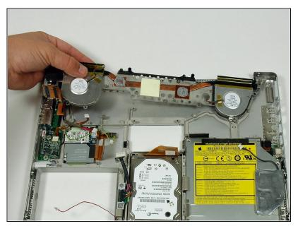
• Lift the heat sink and fans out of the lower case.
