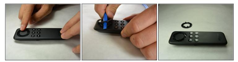
• To remove the buttons use the blue plastic opening tool to pry out the outer ring.
