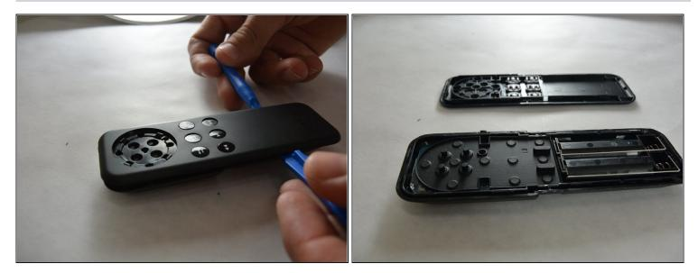
• Remove top plate using plastic opening tools.
