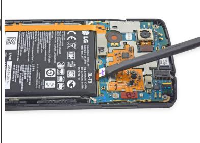
Use the flat end of a spudger to disconnect the battery connector.
