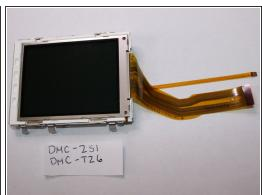
Release the 3 metal clips from the rear cover and remove the LCD
