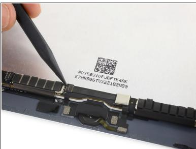
Use the pointed tip of a spudger to flip up the retaining flap on the home button ZIF socket.
