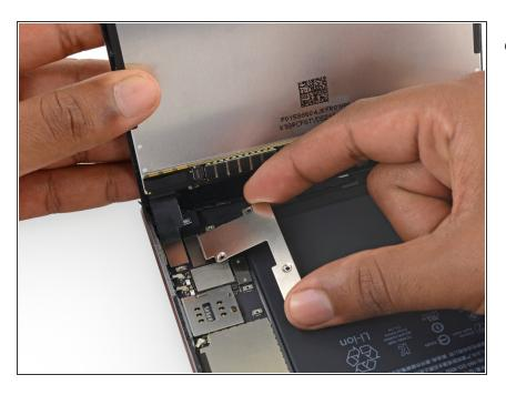
Remove the battery/display cable bracket.
