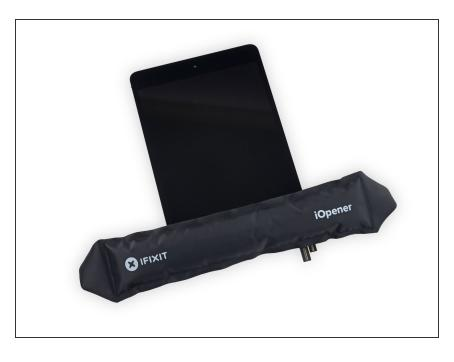
Heat an iOpener and lay it over the lower edge of the front panel to soften the adhesive holding the home button in place.
