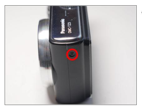
Remove the single .5mm screw on the left side of the camera.
