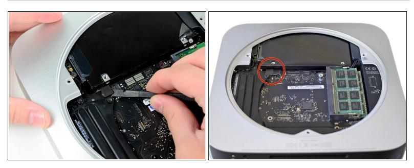
• Use the flat end of a spudger to pry the hard drive connector up from its socket on the logic board.
