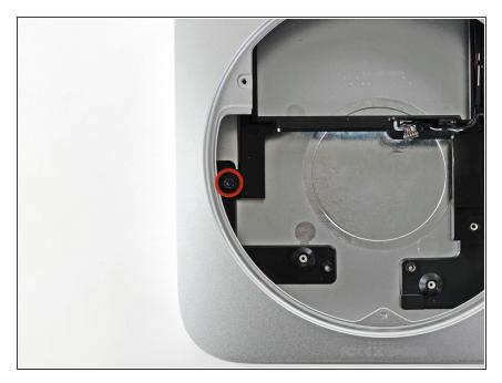
Remove the 7.9 mm T6 Torx screw securing the hard drive tray to the outer case.
