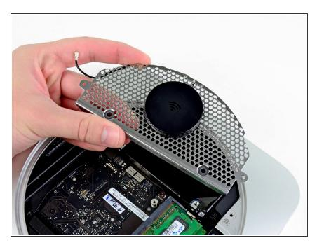
Remove the antenna plate from the mini.
