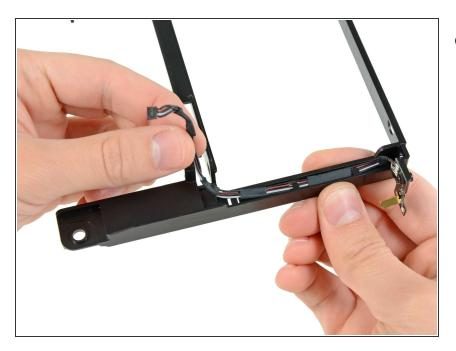
Carefully de-route the IR sensor cables from the channel in the hard drive tray.
