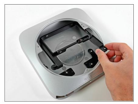
• Remove the hard drive tray from the outer case.
