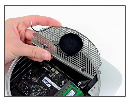
Remove the antenna plate from the mini.
