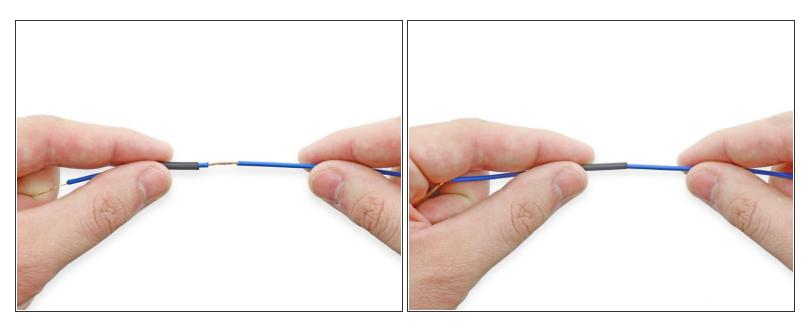
• Slide the tubing onto the wire so that it covers the damaged/exposed section.
