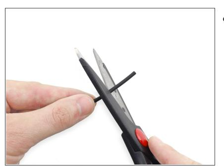
• Use a pair of scissors to cut the tubing to the appropriate length.
