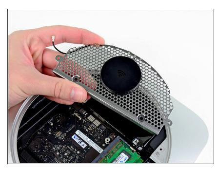
Remove the antenna plate from the mini.
