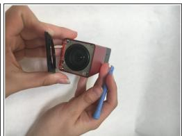
Remove the lens covering by using the plastic opening tool to pry it away from the camera. There
