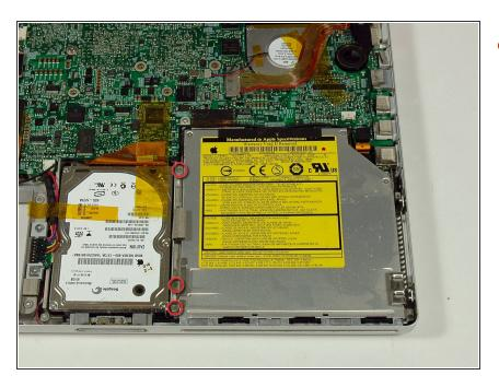
Remove the three 6 mm long silver Phillips screws from the retaining bracket on the left side of the optical drive.
