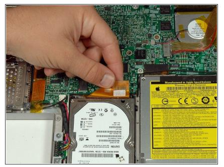
• Disconnect the large orange hard drive cable from the logic board, removing tape as necessary.
