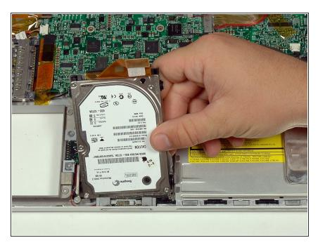
• Lift the hard drive up by the right side and remove it from the computer.
