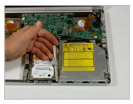
• Remove the retaining bracket.
