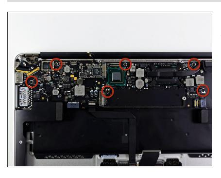
Remove the six 6.3 mm T5 Torx screws securing the logic board to the upper case.
