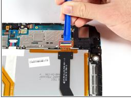
Detach the three connector ribbons passing over the battery using the plastic opening tool.
