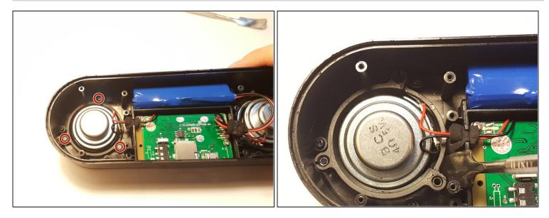
Remove the three screws that are holding the speaker down.
