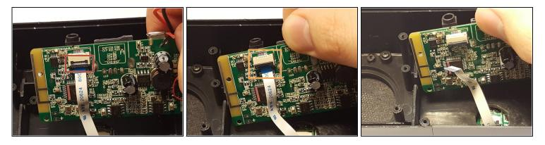
(i) You will finds a ribbon cable connecting the motherboard to the control interface circuit board.
