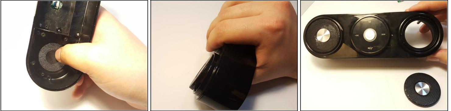
ⓘ Now that the speaker has been removed, the plastic grill should be visible.
