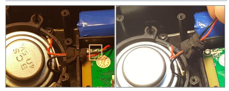
Desolder the speaker joints from the motherboard. Follow this <u>How To Solder</u> guide for help with desoldering.
