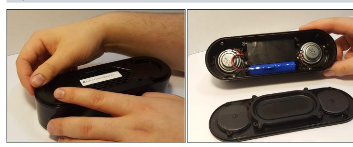
• Remove the bottom panel speaker using an iFixit opening tool.
