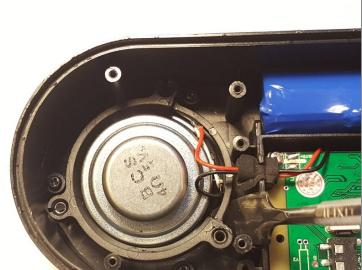
• Remove the three screws that are holding the speaker down.
