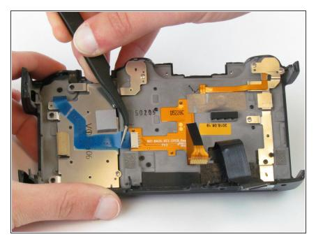
Use the tweezers to pull the blue ribbon cable horizontally out of its clip.
