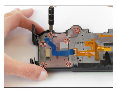
Use the Phillips #00 screwdriver to remove the six screws (three silver 3.5 mm screws and three black 4.2 mm screws).
