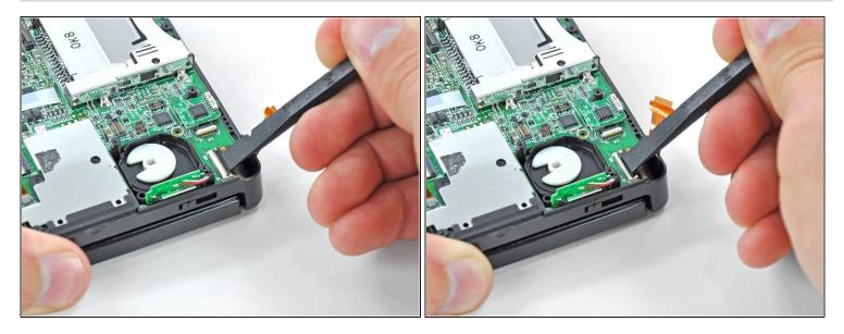
• Use the flat end of a spudger or your fingernail to flip up the retaining flap on the camera ribbon cable ZIF socket.
