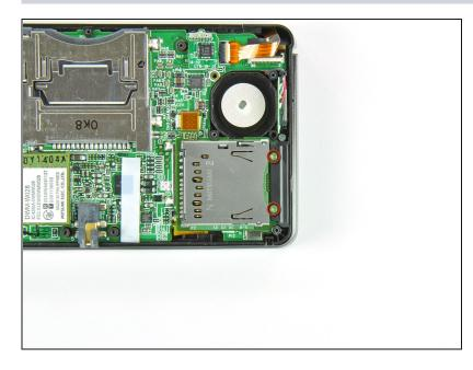
Remove the two 4.5 mm Phillips screws securing the SD board to the motherboard.
