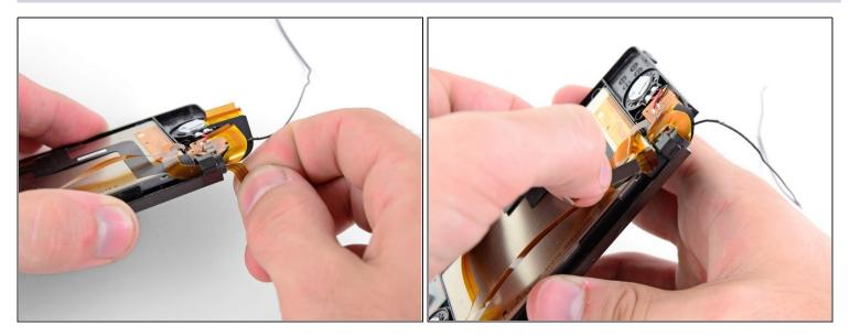
• Carefully feed the speaker assembly ribbon cable through the hole in the upper display bezel.
