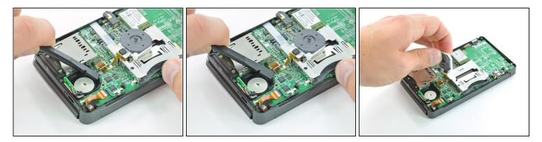
• Use the flat end of a spudger or your fingernail to flip up the retaining flap on the Circle Pad ribbon cable ZIF socket.
