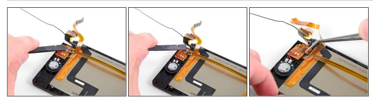
• Use the flat end of a spudger or your fingernail to flip up the retaining flaps on the parallax barrier ribbon cable ZIF sockets.
