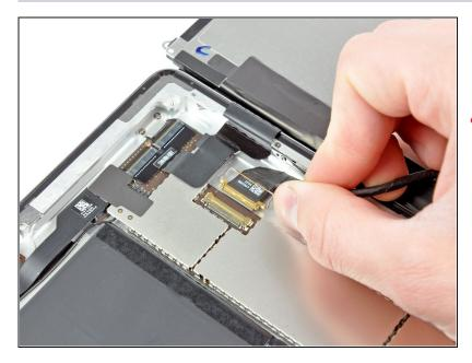
• Pull the display data cable out of its socket on the logic board.
