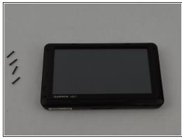
• Remove the four 11.0 mm screws using the Torx T5 screwdriver.
