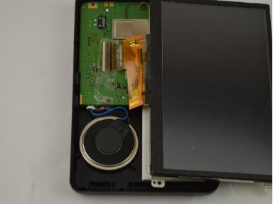
Carefully move the display out of the way of the speaker revealing the blue and black cord from the speaker.
