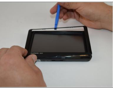
Slide the plastic prying tool around the perimeter to completely remove the frame.
