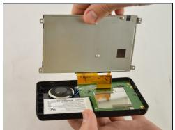
Gently lift up the display screen using your fingers to make sure the only thing connecting it to the body is the ribbon cable.
