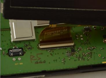
• Remove the piece of tape that is covering the connecting point of the motherboard and display.
