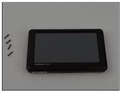
• Remove the four 11.0 mm screws using the Torx T5 screwdriver.
