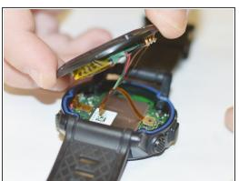
Use a Torx T9 screwdriver to remove these four .8mm screws and seperate the housing.
