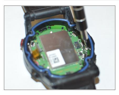
Use your Torx T9 screwdriver to remove the one .8mm screw that holds the main board to the watch housing.
