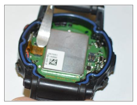
Use a spudger to pry open the power ribbon from the main board.
