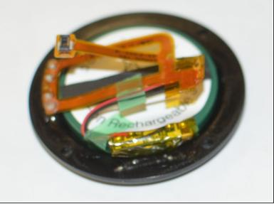
• Use a spudger tool to disengage the power ribbon from the main board. Once the ribbon is disconnected you can separate the bottom piece of the housing that holds the battery.
