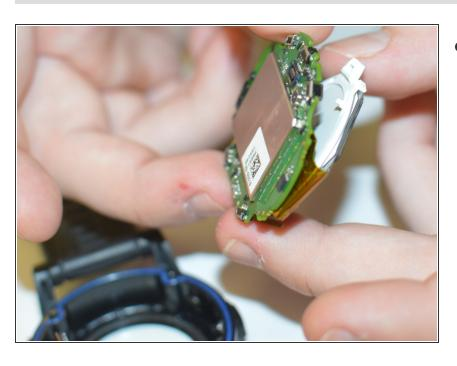
Once removed simply separate the digitizer from the main board.
