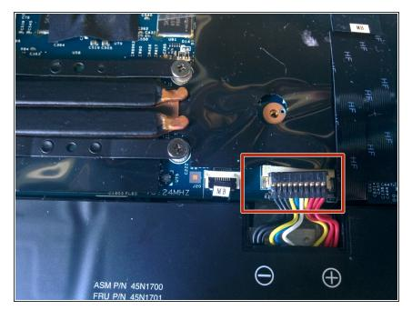
Using a plastic pry tool disconnect the battery from the motherboard.
