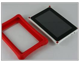
Remove the rubber bumper from the tablet.
