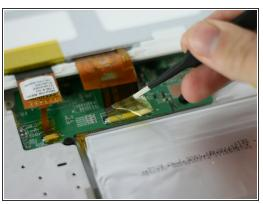
Lay the tablet down flat and remove the yellow tape from the ZIF connector on each side
