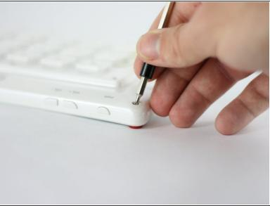
• With a PH00 screwdriver, remove the four outermost screws from the back of the tablet.
