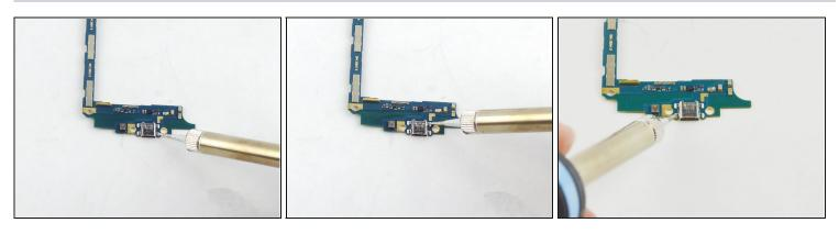
Using a soldering iron to solder off the charging port.
