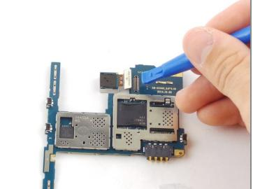
• Remove the motherboard and unhook the ribbon cable clip to the back camera.
