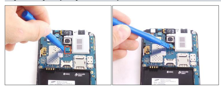
• Unhook the ribbon cable clip with the plastic opening tool and remove the audio jack.
