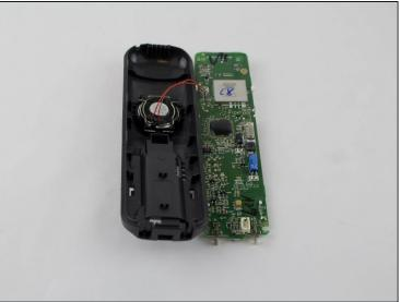
• Remove the two 3.65 mm screws on the motherboard with a PH1 screwdriver.
