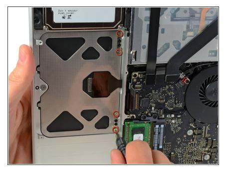
While holding the edge of the trackpad closest to the logic board with one hand, remove the four 1.2 mm Phillips screws highlighted in red.
