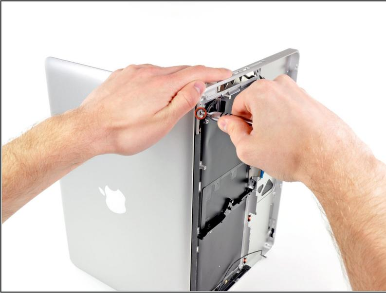
⚠ Be sure to hold the display and upper case together with your left hand. Failure to do so may cause the freed display/upper case to fall, potentially damaging each component.
