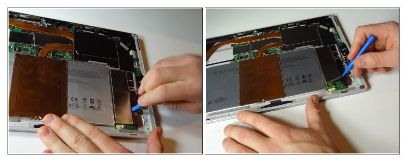
• Use a blue plastic opening tool to pry around the edges of the metal shield covering the SSD drive.
