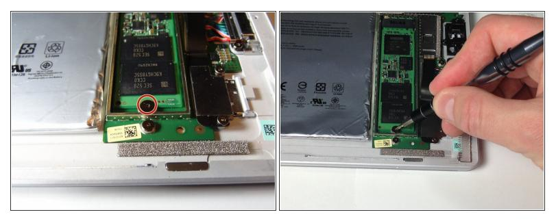
Remove the 1.0 mm Torx T4 screw holding down the SSD drive.
