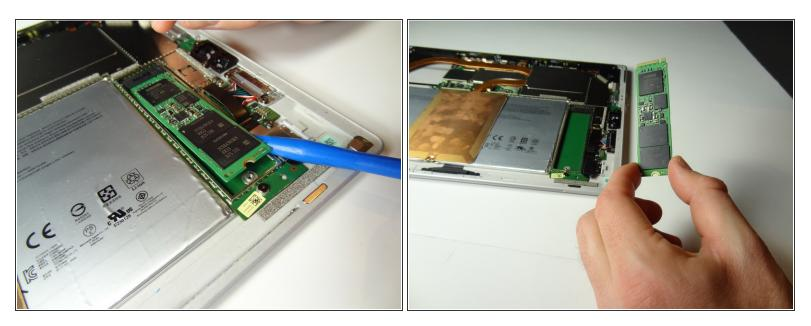
Use a blue plastic opening tool or spudger to lift the SSD drive slightly and grasp it with your fingers. Pull the drive down towards yourself to remove it from the device.
