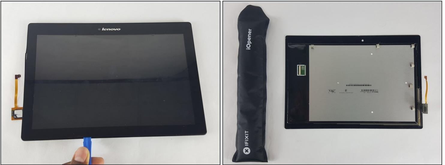
ⓘ The screen is secured by adhesive around all the edges of the screen.
