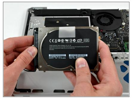
Remove the hard drive from its cable by pulling the cable connector straight away from the drive.
