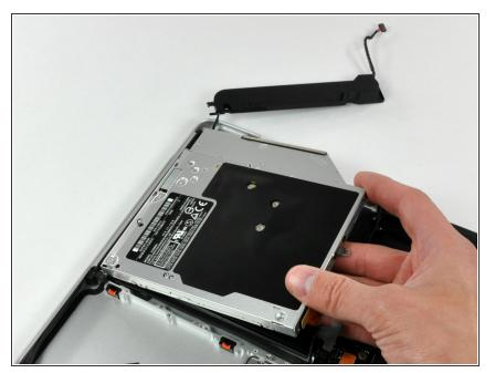
• Lift the optical drive from its right edge and pull it out of the computer.
