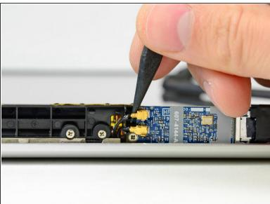
Use the tip of a spudger to pry both AirPort antenna connectors out of their sockets on the AirPort board.
