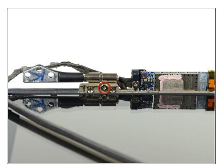
Remove the single 5.2 mm T6 Torx screw securing the right clutch hinge nearest the display glass.
