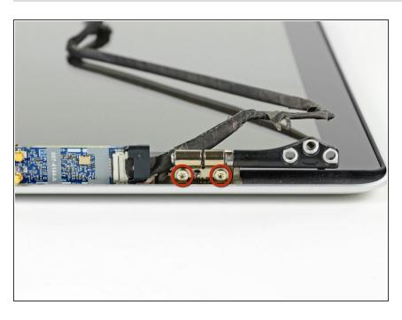
Remove the two remaining 5.2 mm
