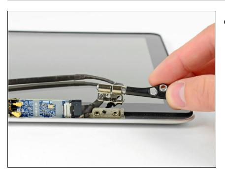
Remove the right clutch hinge.
