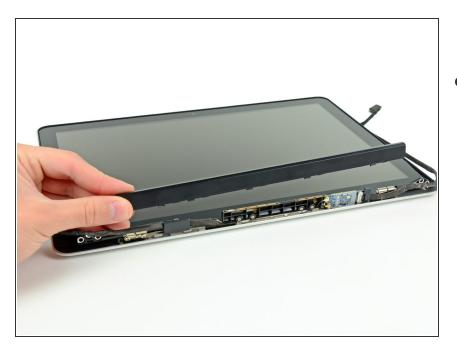
Remove the clutch cover from the display.
